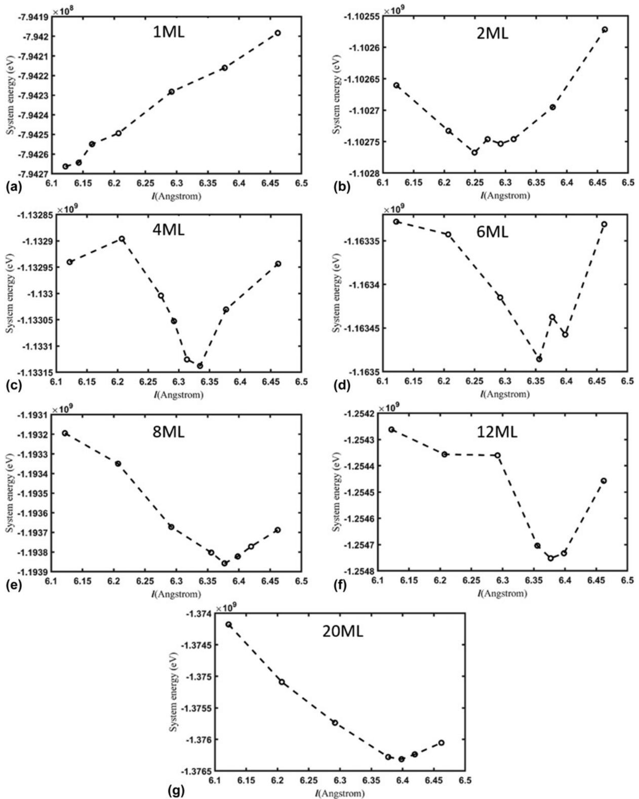
**Figure 1:** Potential energy of relaxed bicrystal models versus distance,  $l$ , of adjacent unit cells in the PbTe layer along the X and Y directions in the initial bilayer models at the layer thicknesses of (a) 1 ML, (b) 2 ML, (c) 4 ML, (d) 6 ML, (e) 8 ML, (f) 12 ML and (g) 20 ML, respectively.
