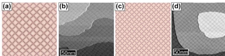
**Figure 3:** Atomic configuration of the PbTe/PbSe interface, (a) and (c) CAC simulation results with the PbTe layer thickness being (a) 4ML and (c) 8ML, respectively; the image size is  $180 \times 180$ ; (b) and (d), STM images of PbTe epilayers on PbSe (001) at coverages of (b) 4.5 ML and (d) 9ML, respectively. (b) and (d) reuse the STM images in Springholz and Wiesauer's paper in 2001 [38].
