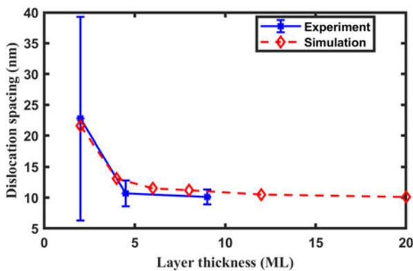
**Figure 4:** The average-dislocation-spacing as a function of PbTe layer thickness. The experimental results [41] are shown for comparison. For 1ML PbTe layer, no misfit dislocations are observed at interface in both CAC simulations and experiments.
