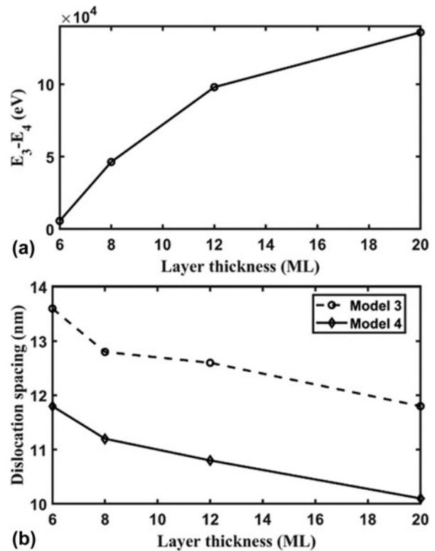
**Figure 5:** (a) The relative potential energy of relaxed configuration of model 3 ( $E_3$ ) with respect to that of model 4 ( $E_4$ ); (b) average misfit dislocation spacings in the relaxed configurations of model 3 and model 4 as a function of layer thickness, respectively.
