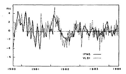
Figure 3. Comparison of UT1 between IMPS optical astrometry and VLBI with respect to BIH UT1 (Yokoyama, 1984).
