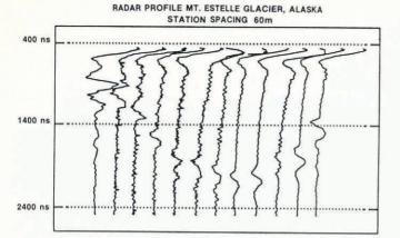
Fig. 4. An ice-radar profile across Mount Estelle glacier as recorded using the PC-based receiver.
