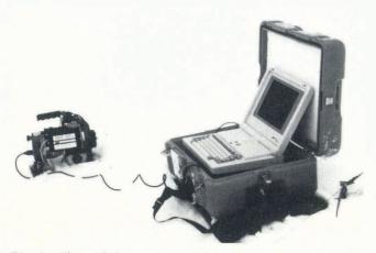
Fig. 1. The PC-based ice-radar receiver in operation on Mount Estelle glacier, Alaska, U.S.A.
