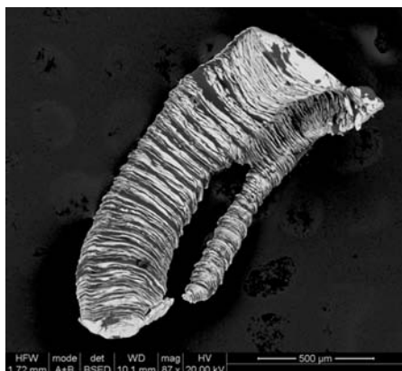
Fig. 4. A BSE-SEM image of a stainless steel fragment with a contaminating partial coating. The fragment has kinked and buckled many times to produce the corrugated appearance.
