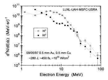
FIGURE 2. Distribution of electrons measured in magnetic spectrometers at 30° (open) and 95° (solid), from the first short-pulse (0.5 ps) petawatt shot series on 5 September 1997. The 0.5-mm Au target was backed by 0.5-mm Cu. The estimated incident laser energy was 280 J, delivered in 450  $\pm$  50 fs, with an estimated focused intensity of  $8 \times 10^{19}$  W/cm<sup>2</sup>.
