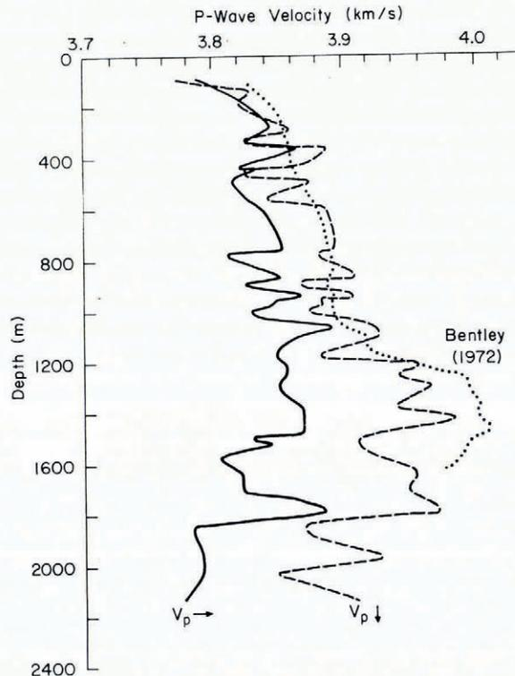
Fig. 2. Axial ( $V_{p\downarrow}$ ) and diametral ( $V_{p\rightarrow}$ ) ultrasonic P-wave-velocity profiles for ice cores from Byrd Station deep drill hole. Bentley (1972) velocity profile was obtained from measurements along bore-hole axis. Note that  $V_{p\downarrow}$  is parallel to the bore-hole axis.
