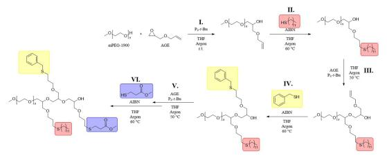
**Scheme 1.** The overall synthetic scheme of the anionic ring-opening monomer addition of AGE to mPEG-1900 to synthesise sequence-controlled polymers. The individual steps of chain extension (I., III., and V.) and post-polymerisation modification (II., IV, and VI.) reactions are displayed.
