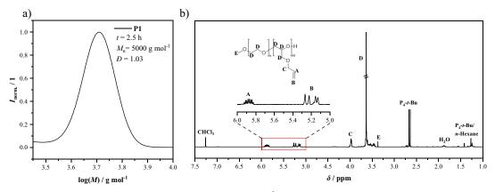
Figure 1. (a) Size exclusion chromatogram and (b)  ${}^{1}H$  NMR spectrum (solvent: CDCl<sub>3</sub>) of P1.
