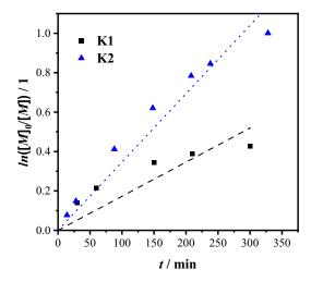
*Figure 2. Kinetic study of the polymerisation of AGE using non-treated (K1; blue) and dried (K2; black) mPEG-1900.*
