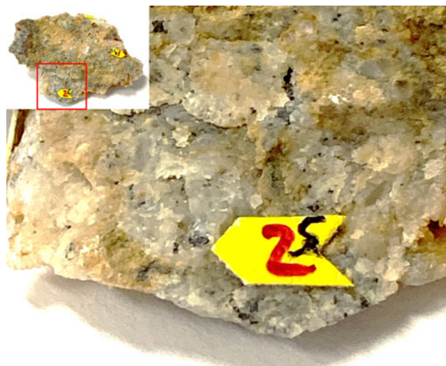
Figure 2. Argentopolybasite- 72ac -bearing specimen (6 cm wide) from the IXL mine, Silver Mountain mining district, Alpine County, California. The specimen also contains pyrite, argentepearceite and acanthite.
