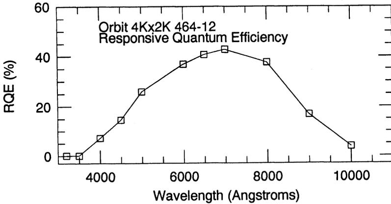
Fig. 3. Measured RQE for for thick 4k x 2k CCD
