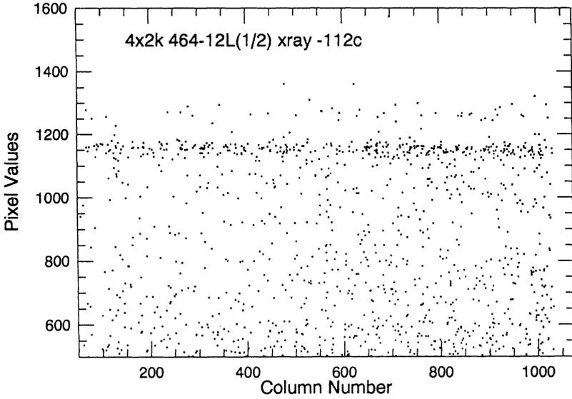
Fig. 1. CTE measured using Fe-55 X-rays
