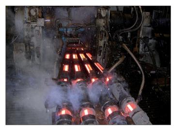
Siemens will supply the mechanical process equipment, a re-heating furnace, a water treatment plant, the fluids systems, and the complete electrical and automation equipment.
