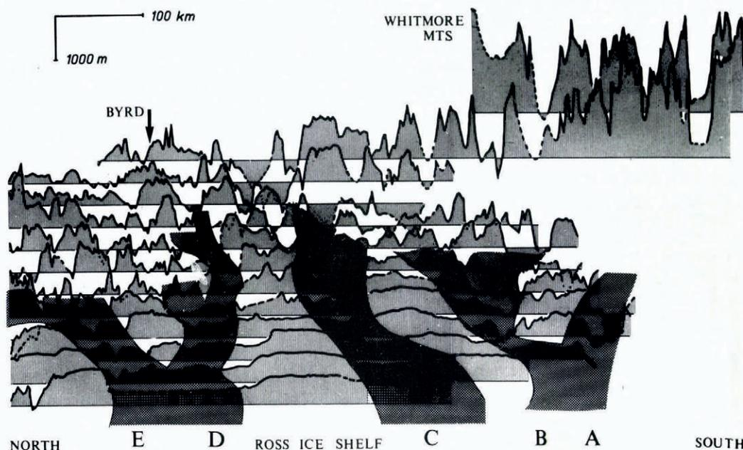
Fig. 2. Radio-echo profiles of bedrock at 50 km spacing traversing Marie Byrd Land parallel to long.  $135^{\circ}$  W. The common datum for profiles, the base of the shading, is at  $-1\ 000$  m. The effective separation is 500 m. Positions of ice streams are shown by the heavier sections of profiles and the stippling. Interpolated data are represented by dashes. Dots show obscured sections.
