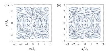
FIGURE 3. (Colour online) Streamlines of the isothermal heat flux generated by a point force at the origin (note,  $\theta = 0$ ): a comparison of the Gradlet (a, equation (2.22)) and the Reglet (b, equation (2.33)). Plots are in a plane containing the point force (z = 0), with a range  $\pm 2.7\lambda_e$  in the x and y directions. The bold arrow indicates the direction of the point force.
