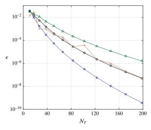
FIGURE 7. (Colour online) Numerical error of Gradlet–MFS drag prediction,  $\epsilon$ , against number of boundary nodes, N. Four singularity site distributions are used: sites located on the surface of an origin-centred sphere with radius a=0.2 (-\*-), a=0.3 (-o-) and a=0.4 (- $\Delta$ -); and sites located on the surface of a sphere centred at  $\mathbf{x}=[0.1,0,0]$  with radius a=0.2 (-+-).
