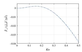
FIGURE 11. (Colour online) Total non-dimensional force on identical, adjacent and stationary spheres generated by a difference in sphere temperature  $(\Delta \hat{\theta})$ , against Knudsen number (based on sphere radii). Gradlet–MFS solutions with N=132 (--), N=204 (—) and N=292 (···) total boundary nodes.
