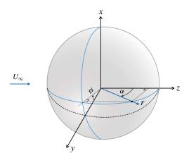
FIGURE 5. (Colour online) Coordinate system for flow around a sphere:  $\alpha$  is the polar angle,  $\phi$  is the azimuthal angle and  $r = \|x\|$  is the radial coordinate. Flow direction is in z, and the sphere is centred at the origin, with its boundary at r = 1 (non-dimensionalisation is performed with the sphere radius  $\hat{a}$ ).
