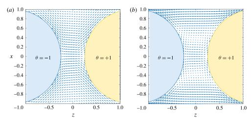
FIGURE 10. (Colour online) Velocity field (at y=0) generated between stationary spheres having a fixed and uniform temperature difference: (a) Kn=0.1; (b) Kn=0.5. See figure 9 caption for other details. Glyph lengths are normalised to the maximum velocity magnitude for each figure.
