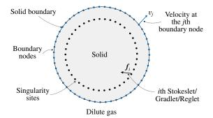
FIGURE 4. (Colour online) Illustration of the method of fundamental solutions (MFS).
