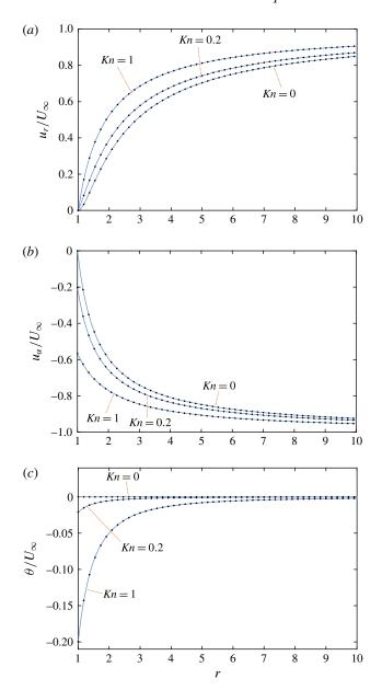
FIGURE 6. (Colour online) Radial variation of: (a) radial velocity at  $\alpha=0$ ; (b) polar velocity at  $\alpha=\pi/2$ ; and (c) temperature at  $\alpha=0$ . Comparison of Young's analytical solution ( $\cdot$   $\cdot$ ) to the Gradlet-MFS solution with N=66 boundary nodes (—), for three Knudsen numbers (Kn=0, 0.2, and 1). Note, the surface of the sphere is at r=1 and all plots are non-dimensional and normalised with the far-field velocity  $U_{\infty}$ .
