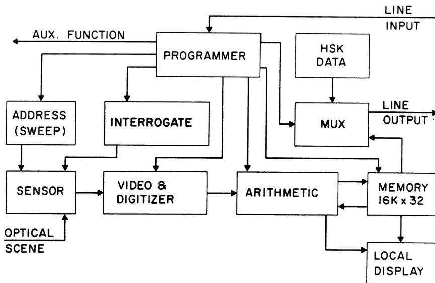
Fig. 2. Real time solar magnetograph, block diagram of electronics, located near the telescope.
