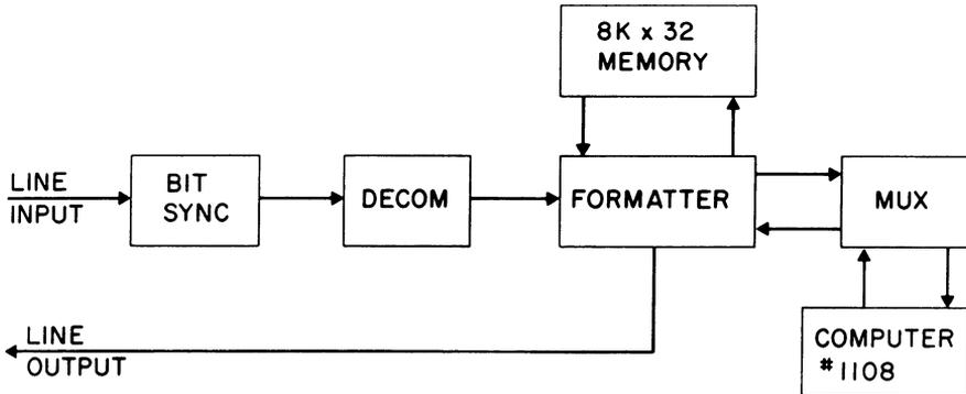
Fig. 3. Real time solar magnetograph, block diagram of electronics, located near the computer.
