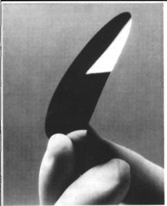
A 3" diameter 2-4 μ membrane manufactured at Virginia Semiconductor, Inc.
