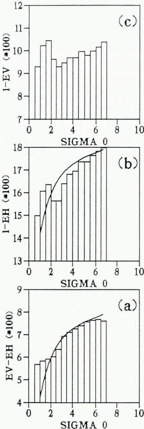
Fig. 5. Empirical relation between the altimetric back-scatter coefficient, averaged over each 0.5 dB interval and (a)  $ev-eh$ , (b)  $l-eh$ , (c)  $l-ev$ , where  $ev$  and  $eh$  are the emissivities in vertical and horizontal polarizations. The theoretical surface-roughness effect on the emissivity (Equations (10)–(12)) are superimposed. The roughness parameter  $S^2$  is deduced from  $\sigma_0$  of the Seasat altimeter (Equation (2)).
