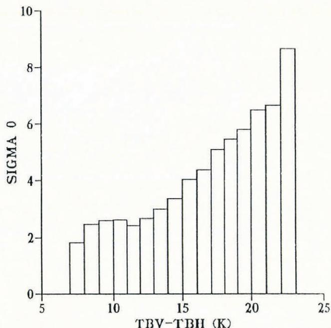
Fig. 4. Empirical relation between  $\sigma_0$ , the altimeter backscatter coefficient and the difference between vertical and horizontal polarizations of the brightness temperatures, averaged for each 1 dB interval of  $\sigma_0$ .  $\sigma_0$  is related to AGC by Equation (1).
