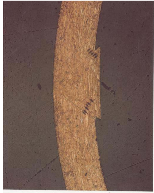
Photograph 4 Adiabatic Shear in 5.56mm Cartridge Brass 70:30 Center Fire Case (Magnification: 75X)
