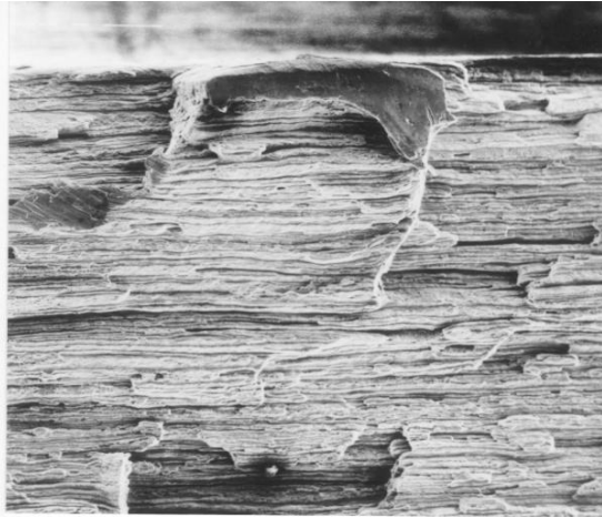
Photograph 1 Fibrous Characteristic of Transverse Crack (Magnification: 100X)
