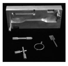
Figure 1. Examples of titanium components fabricated using the aromatic powder injection molding (PIM) binder system.
