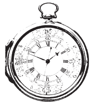
Figure 1.2 Harrison's H4. The first clock able to keep accurate time at sea, enabling determination of longitude.
