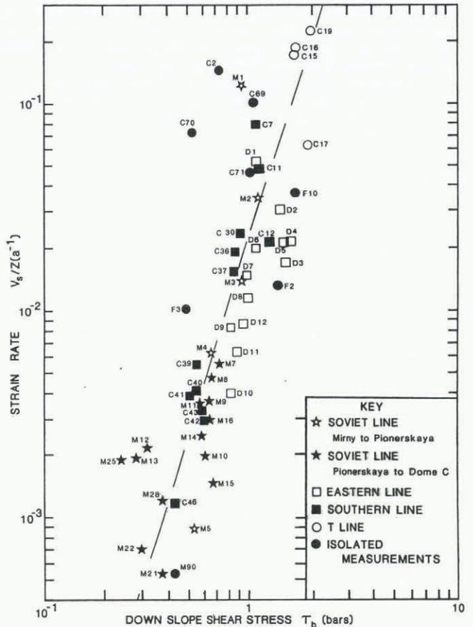
Fig. 6. Strain-rate versus down-slope shear stress with regression line shown dotted. Station names GF10, GM05, etc. are labelled F10, M5, and so on.
