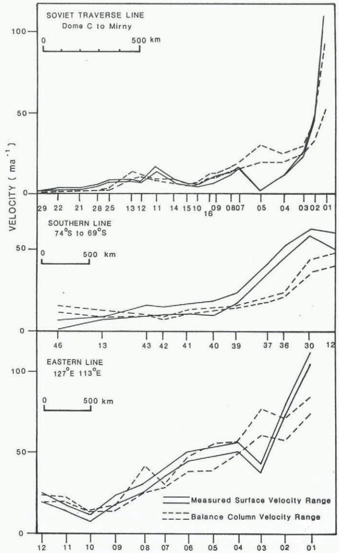
Fig. 2. Velocity profiles along sections of major traverse lines. Location of individual measurements is indicated along with station numbers.
