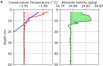
Fig. 10. (left) Schematic of frazil formation at depth during katabatic wind events. (right) Example temperature and salinity profiles from a CTD station in a katabatic wind event in TNBP. Shaded regions show the temperature and salinity anomaly compared to the baseline values (dotted line) where frazil ice is forming and releasing heat and salt. The blue line is the calculated freezing temperature (De Pace and others, 2019).
