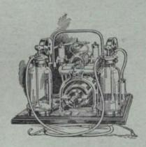
The outstanding feature of this apparatus is that there are two separate pairs of cylinders for pressure and for suction, without intercommunication between them; so the pressure cylinders cannot possibly become contaminated by anything that has been drawn away from any patient.
