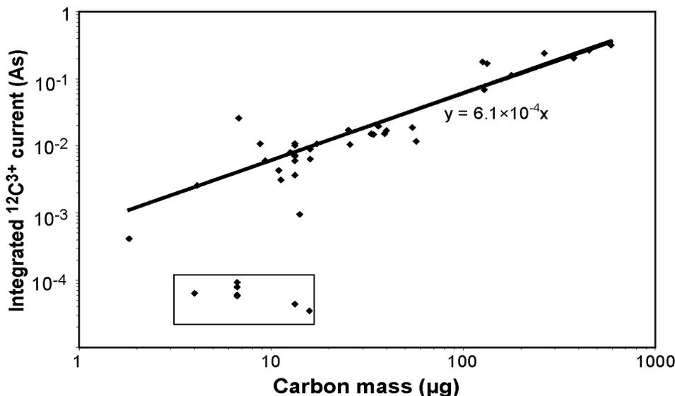
Figure 5 Indication of the analytical sensitivity of graphitization and AMS measurement. The integrated  $^{12}\text{C}^{3+}$  current is shown for all completely sputtered samples versus the carbon mass calculated from the  $\text{CO}_2$  pressure before graphitization. The slope of the linear fit corresponds to a total detection efficiency of 2.1%. The deviating data points in the box are discussed in the text.
