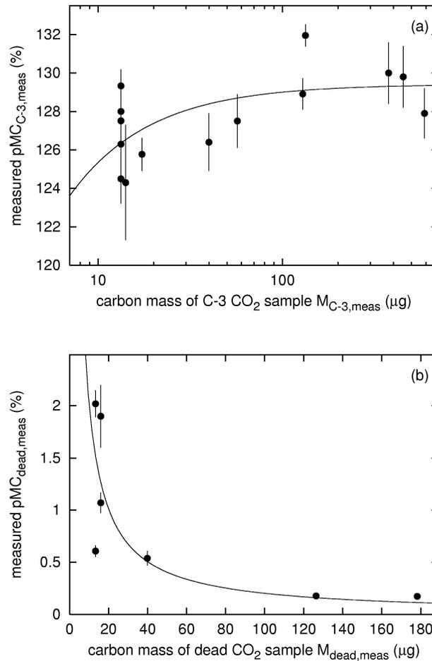
Figure 4 Contamination during CO<sub>2</sub> graphitization and AMS measurements. Measured pMC values for a) IAEA C-3 CO<sub>2</sub> and b) dead CO<sub>2</sub> are plotted versus carbon mass of processed CO<sub>2</sub>. Note that contamination with unknown pMC leads for small standard amounts to measured pMC values that are too low (a). For small blanks, the measured pMC values are too high (b). The curves shown are model fits that allow one to assess the carbon contamination.
