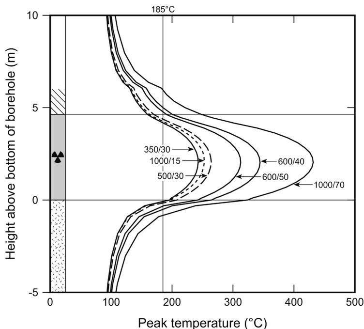
FIG. 4. Examples of peak temperatures at the outer surfaces of single containers. The short dashed line is for UO<sub>2</sub>-65, the long dashed line for MOX-55 and the solid lines for MOX-65; arrows indicate the number of pins per container and the age of the fuel (years).
