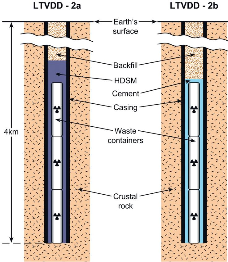
FIG. 1. Deep borehole disposal concepts LTVDD-2a and LTVDD-2b showing alternative support matrices (not to scale).
