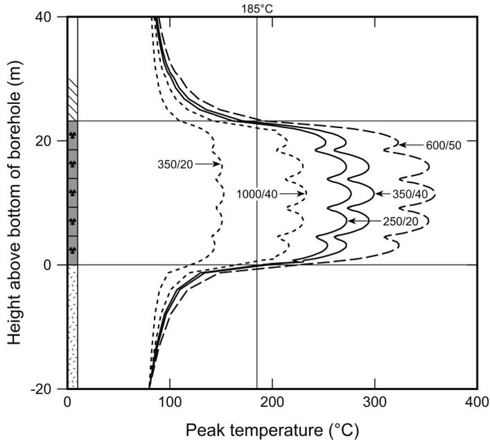
FIG. 8. Examples of peak temperatures at the outer surfaces of the containers in batches of 5 emplaced at 7 day intervals. The short dashed lines are for  $\text{UO}_2$ -65; long dashed line is for MOX-55 and solid lines are for MOX-65; arrows indicate the number of pins per container and the age of the fuel (years).
