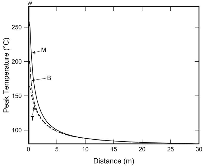
FIG. 5. Peak temperatures along horizontal radii out into the host rock for a single container with 1000 pins of 15 year old  $UO_2-65$ . Abbreviations used are T, top of the container; M, middle of the container; B, bottom of the container; and W, borehole wall.
