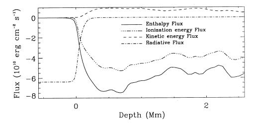
Fig. 9. Radiative, enthalpy (convective), ionization energy (latent heat) and kinetic energy fluxes as a function of depth.
