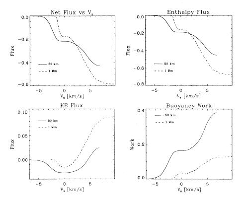
Fig. 10. Net flux, enthalpy flux, kinetic energy flux and buoyancy work at 50 km and 1 Mm depth as a function of fluid velocity. The fluxes and work are summed over area for fluid velocities ranging from maximum upflow to maximum downflow.
