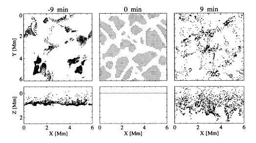
Fig. 3. The origin and destination of fluid parcels ascending through the visible surface at time t = 0. Nine minutes earlier, most of these parcels originated from a small source volume – vertically (because they have nearly the same vertical velocity) and horizontally (because the upflow diverges). Nine minutes later, most of the fluid has descended a substantial distance, concentrating into a few filamentary downdrafts.
