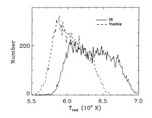
Fig. 14. Histogram of the radiation temperature at 0.63 and 1.6  $\mu$ m. The average radiation temperature is 6047 K at 0.63  $\mu$ m and 6352 K at 1.6  $\mu$ m. The rms relative radiation temperature fluctuation is 0.036 at 0.63  $\mu$ m and 0.043 at 1.6  $\mu$ m.
