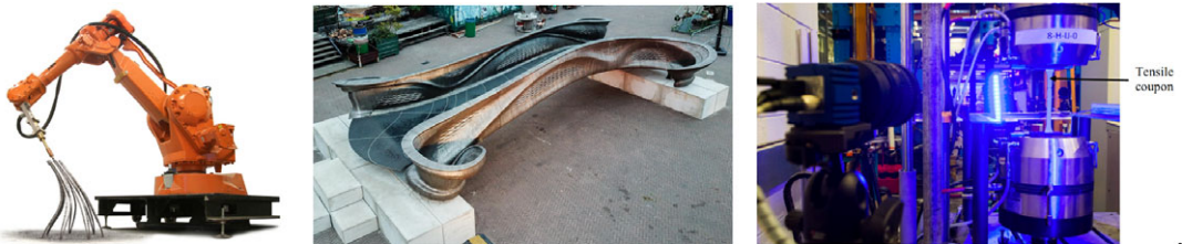
Figure 5. (Left) The 3D-printing protocol developed by MX3D uses a weld head attached to a robotic arm (image by Joris Laarman, www.jorislaarman.com ). (Middle) Pedestrian bridge manufactured using 3D-printed steel (7). (Right) Test set of up of individual coupons.
