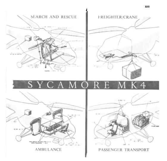
The basic Sycamore helicopter is provided with all the fixed fittings needed to convert it to any of the four major rôles for which it is primarily designed. To equip the basic aircraft for any one of the rôles, or to change it from one to another, is a simple operation needing no elaborate equipment or special facilities
