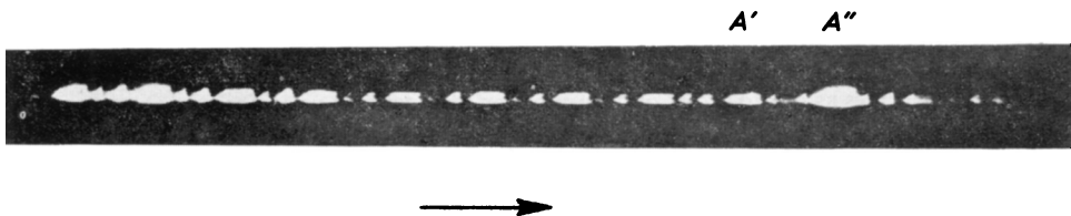
FIG. 1. The image of a meteor photographed on August 8, 1965, through a rotating shutter with three different open sections. The triangular form of the segments of the meteor path is due to diffraction effects. Note that the distances between the fainter and the mean segment are almost constant up to the point A' , but then this distance increases instantaneously. A new fragment has appeared between A' and A'' , and after the point A'' it becomes bright. This means the division of the body into two objects.
