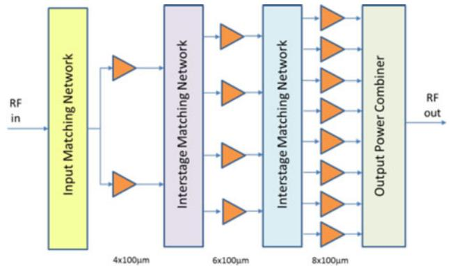
**Fig. 5.** Architecture of the HPA MMIC. For the networks, it has been preliminary estimated a power loss of 1 dB for the output combiner and 1.5 dB for both the interstage matching networks.
