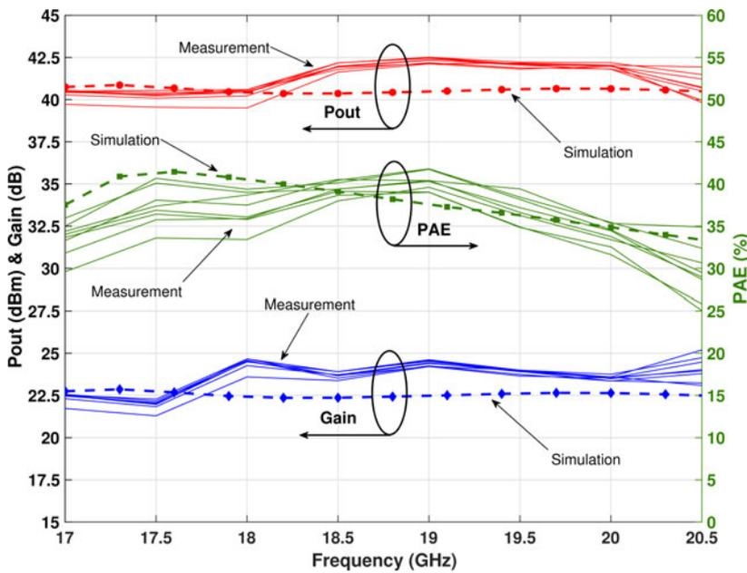
Fig. 18. Comparison between simulated (dashed lines) and measured (continuous lines) power performances. The latter refers to the same MMIC version located in different wafer positions, to test the reproducibility of the results on the wafer.
