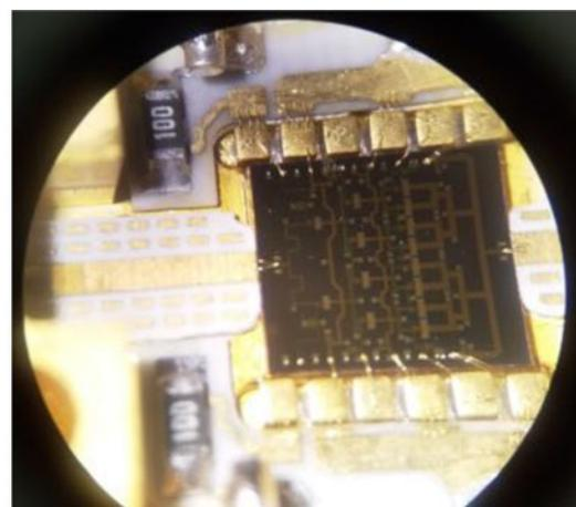
Fig. 19. (a) MMIC mounted in the package. (b) Zoom on the MMIC area.
