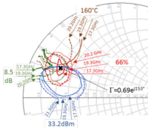
**Fig. 2.** Load pull for the  $8 \times 100 \mu\text{m}$  device for the carrier frequencies of 17.3, 19.3, and 20.2 GHz. The input power is 24.7 dBm. The blue contours refer to the output power, green to the gain, red and brown to the drain efficiency and junction temperature, respectively.
