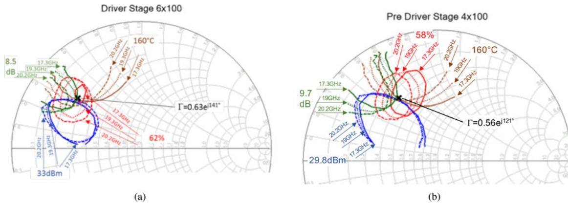
**Fig. 8.** Simulated load pull for the devices used in the driver (a) and pre-driver (b) stages. The former is  $6 \times 100 \mu\text{m}$ , the latter  $4 \times 100 \mu\text{m}$ , both biased with  $V_{DD}=11.25\text{ V}$  and quiescent current  $I_D=27\text{ mA}$  and  $I_D=18\text{ mA}$ , respectively. The contour plots refer to 1 dB of gain compression.
