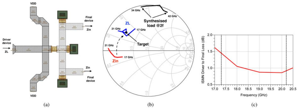
**Fig. 9.** Designed interstage matching network between driver and final stages (a) and synthesized load (b). The insertion loss is within 1 and 1.5 dB (c). (a) Interstage matching network between one driver and two final devices. (b) Synthesized loads. (c) Combiner loss.
