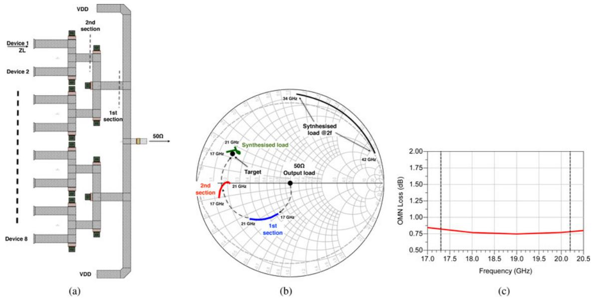
Fig. 6. Designed output combiner (a) and synthesized load (b). The power losses result in ~0.8 dB (c). (a) Output combiner. (b) Synthesized loads. (c) Combiner loss.
