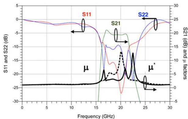
**Fig. 13.** Simulated small-signal S-parameter.
