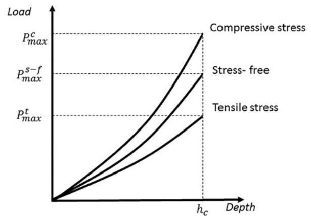
**Figure 1:** Schematic load–depth curves for indentation loading, comparing stressed sample and stress-free sample.
