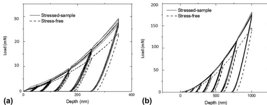
**Figure 5:** Load–displacement curves for 9 indents on the shot-peened sample (solid lines) and the corresponding single indentation on a sample prior to peening (dashed line) to (a) maximum indentation depth 350 nm, (b) maximum indentation depth 1000 nm. Note the stress relaxation during the hold overlaps on the 9 indentations; the magnitude of stress relaxation for any single indent is similar between the stressed and stress-free cases.
