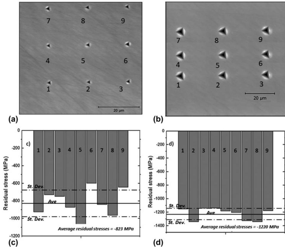
Figure 6: Residual stresses corresponding to the indentation on the shot-peened surface obtained by energy model, (a and c) maximum indentation depth 350 nm, (b and d) maximum indentation depth 1000 nm.
