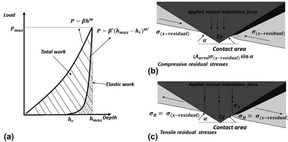
**Figure 2:** Load displacement curve and residual stress state, (a) comparing elastoplastic energy area under loading unloading curve, (b) schematic compressive residual stress state at the indentation surface, (c) schematic tensile residual stress state at the indentation surface.
