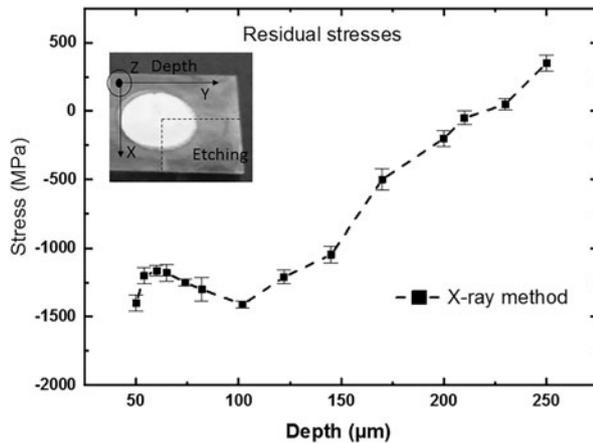
**Figure 4:** X-ray residual stress measurement on the corresponding depth with electro-etching method. Error bars the represent instrument precision.
