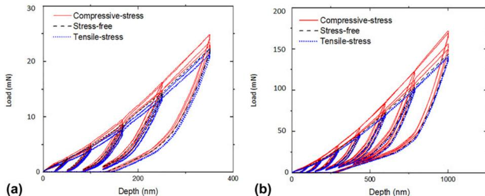
Figure 7: Loading and unloading curves for stressed and stress-free samples on the cross section, (a) indentation depth 350 nm, (b) indentation depth 1000 nm.
