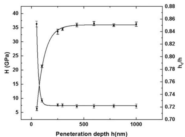
**Figure 3:** Experimental determination of size effect (hardness as a function of depth) and contact depth to penetration depth ratio obtained from multiple cycles of single indentations. Error bars represent standard deviation of 5 indentations, points represent the mean of 5 measurements.
