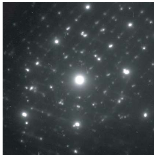
FIG. 3. Selected Area Diffraction Pattern of rapidly solidified Al_{40}Cu_{10}Mn_{25}Ge_{25} exhibiting five fold symmetry.
