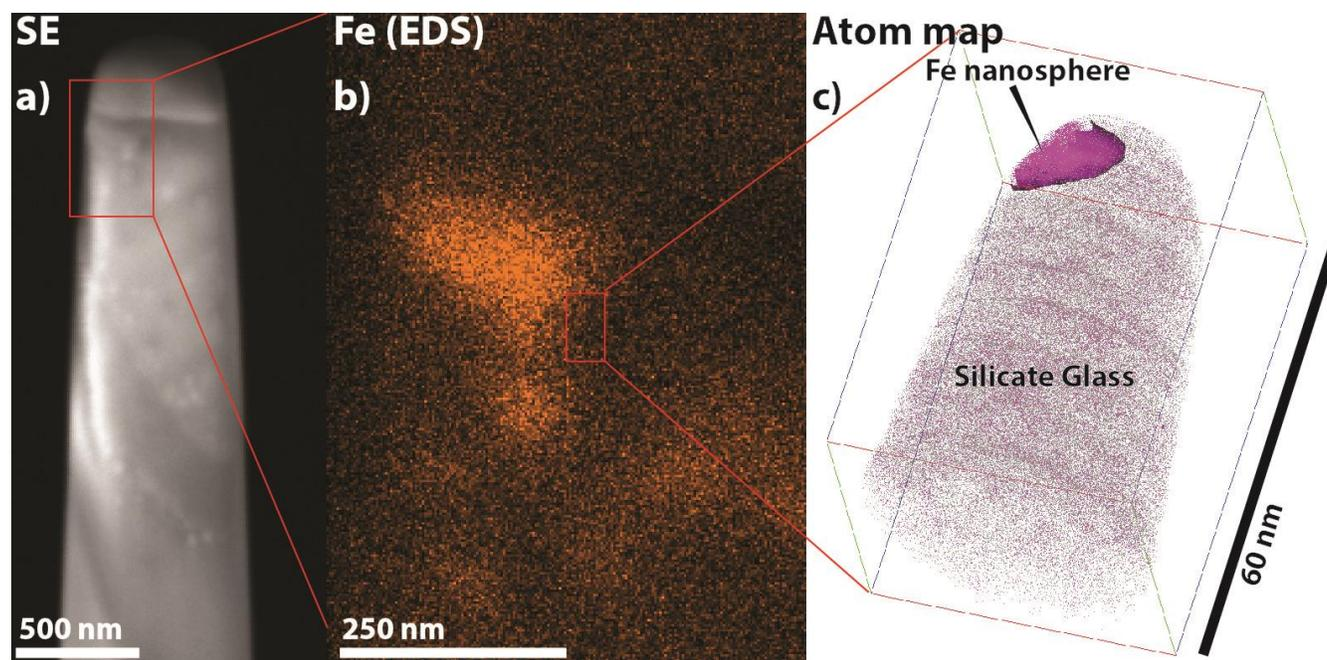
**Figure 1.** (a) SE image of atom probe needle prior to final polishing, red box is area enlarged in figure 1b.
