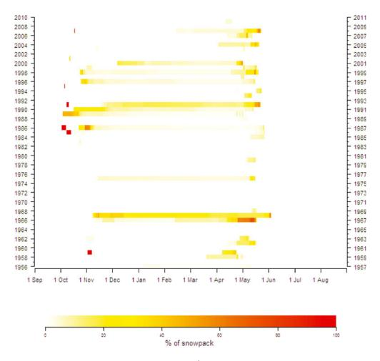
Fig. 6. Percentage of total snow depth having density above 350 kg m<sup>-3</sup> for the hydrological years 1956–2010 (1 September–31 August).
