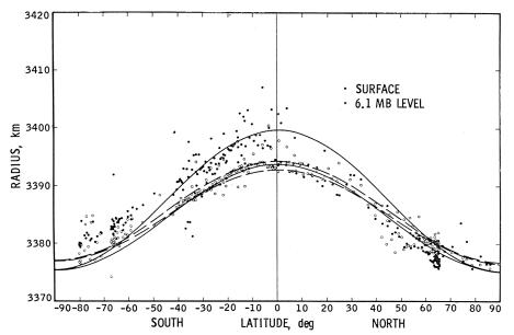
Fig. 17. Occultation radii measured by Mariner IX. The closed circles indicate radii of the solid surface and the open circles are derived radii of the 6.1 mb pressure level. The solid and dashed lines define the radii of fitted tri-axial ellipsoids approximating the solid surface and a 6.1 mb isobaric surface, respectively.
