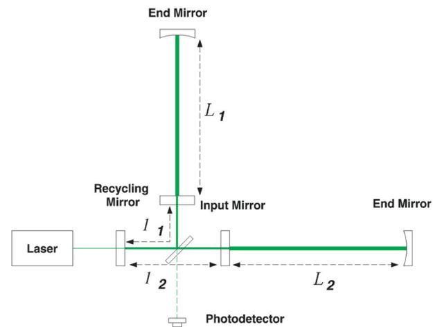
**Figure 1** Optical layout of first-generation long baseline interferometers.
