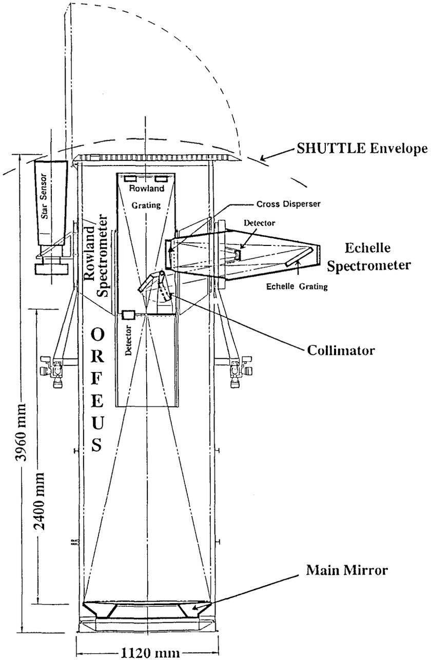
Fig. 2. Cross Section of the ORFEUS telescope system.
