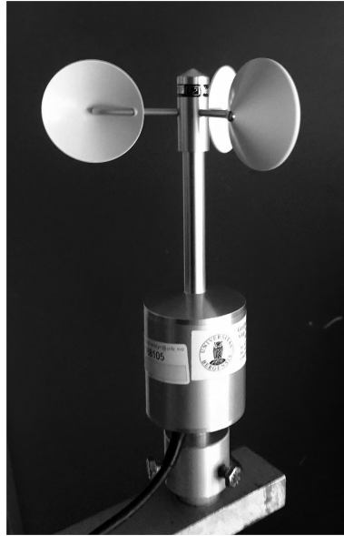
Figure 2.18 Cup anemometer with three cups. Photo by Stephan Kral, University of Bergen.
