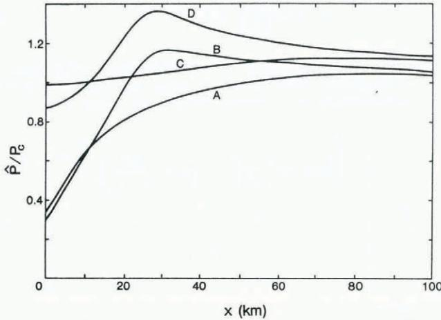
Fig. 4. Ratio of  $\hat{P}(x)$  (Equation (30)) to  $P_c(x)$  (Equation (14)). Curves C and D use  $\hat{Q}$  from Equation (26). Curves A and B use  $\hat{Q} = Q$  from Equation (24) (winter).  $\kappa$  values are 1.2, curves A and C, and 2.0, curves B and D.
