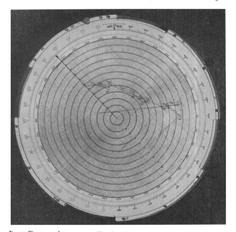
Fig. 1. The compass-datum computer. The relative bearing (outer) ring may be turned to set ship's head to any desired point on the compass course or bearing scale and then clamped. The compass scale is fixed to the plotting surface. The graticule with its pointer is on a disk which may be turned independently of either bearing scale. The computer, being circular, may be held with either ship's-head or north  $(000^\circ)$  upwards, according to preference.
