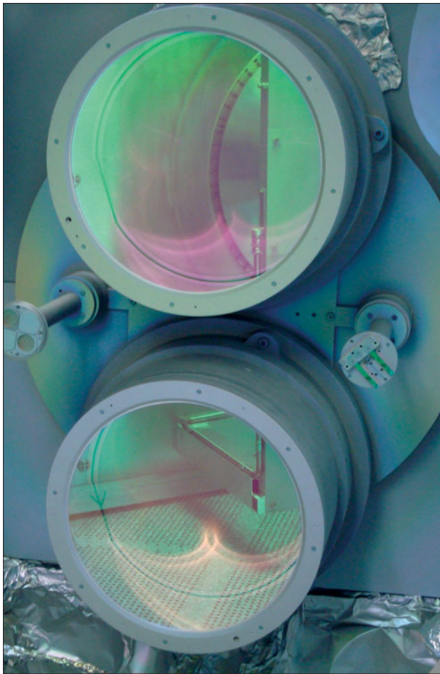
Two LIGO test masses after coating in the ion-beam sputtering deposition chamber at the Laboratoire des Matériaux Avancés (LMA) in Lyon, France. Credit: LMA.
