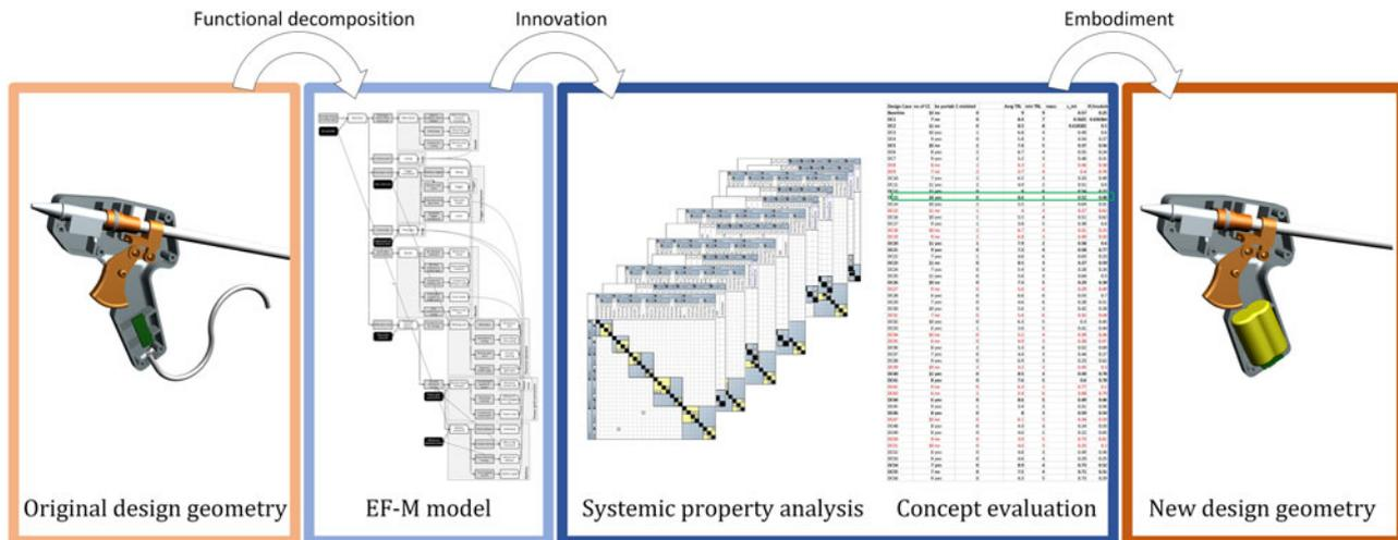
**Fig. 6.** Visualization of the concept evaluation process; EF-M model containing all variants, DSM derived from the EF-M model, table of 56 concepts and evaluation criteria with the baseline highlighted in blue and the chosen concept in green, renderings of baseline and chosen concept.
