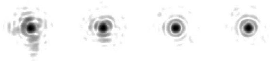
**Figure 2.** PSF corresponding to the 4 first points of Fig 1, represented in invert logarithmic scale. The PSF on the left is the PSF obtained without any pre-compensation and used to perform the first PD measurement (iteration 0). The 3 other PSF correspond to iteration 1, 2 and 3 respectively.  $\lambda = 632nm$ .
