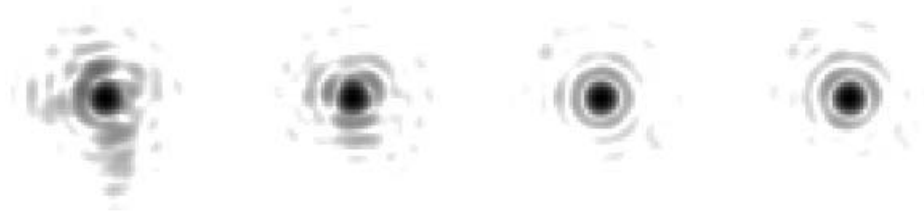
Figure 2. PSF corresponding to the 4 first points of Fig 1, represented in invert logarithmic scale. The PSF on the left is the PSF obtained without any pre-compensation and used to perform the first PD measurement (iteration 0). The 3 other PSF correspond to iteration 1, 2 and 3 respectively. \lambda = 632nm .
