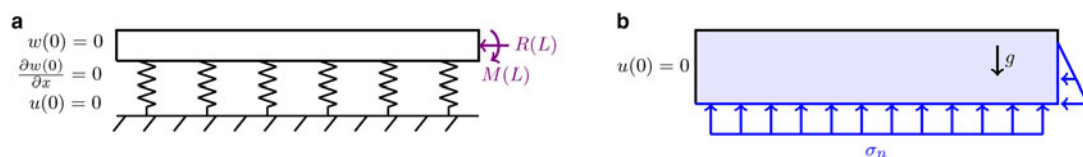
Fig. 2. (a) Boundary conditions for the beam theory used in Reeh (1968). (b) Boundary conditions for the 2-D continuum approach using finite element simulation.
