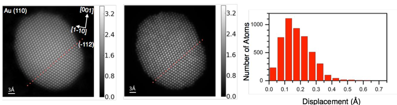
**Figure 1.** Experimentally measured STEM image of Au nanoparticle (left); Simulated STEM image of the GA optimized structure (middle); Comparison of atomic column displacements between experiment and simulation (right).
