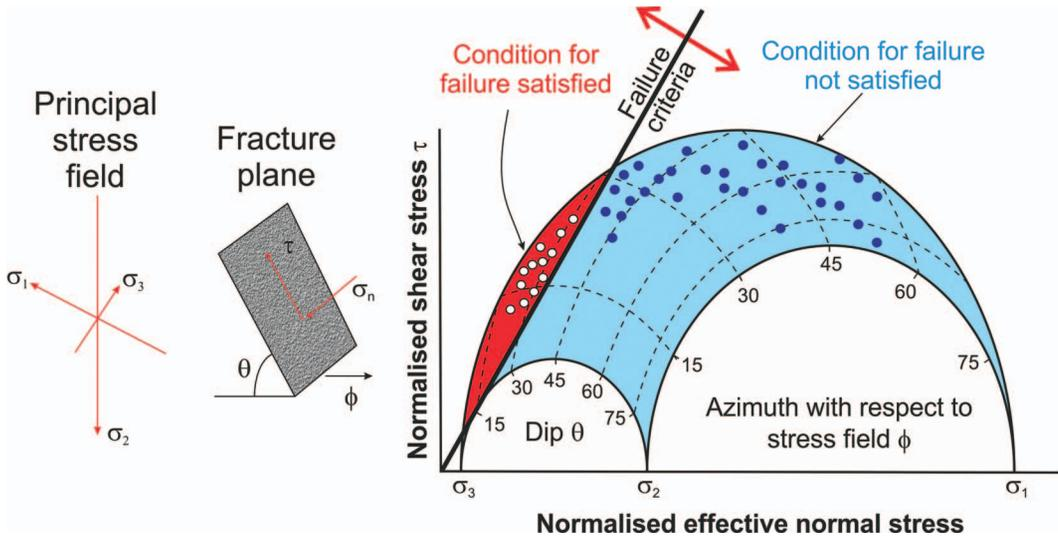
FIG. 1. Critical stress hypothesis (adapted from Barton *et al.*, 1995; Jaeger *et al.*, 2007; Rogers, 2003). The three-dimensional Mohr diagram represents the shear stress and normal stress acting along a fracture in response to the *in situ* stress field. The open circles represent fractures experiencing state of stress above the failure criterion and therefore subject to shear failure. The closed circles represent fractures for which the stress state is insufficient to induce shear failure.
