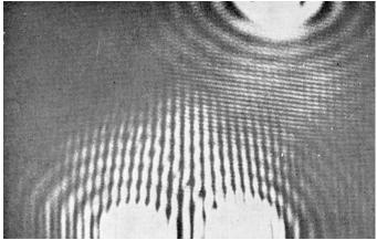
This picture, taken from Jesper Munch's thesis and analogous to a Young double slit interference pattern, was produced by electrons passing through minute holes in a gold film.
