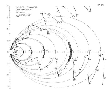
Fig. 2. Time-labeled trace of Pioneer ll's encounter trajectory on a magnetic meridian plane through the spacecraft. The assumed Jovian dipolar model is specified. The cross-hatching shows the regions that bound the orbits of JV (Amalthea), JI (Io), JII (Europa), JIII (Ganymede), and JIV (Callisto) in this coordinate system. The time is "Earth Received Time" as in Figure 1.
