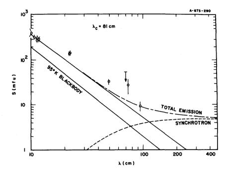
Fig. 12. Observed values of radio spectral power flux from Saturn and an illustrative example of the synchrotron contribution from a hypothetical radiation belt of relativistic electrons (Luthey 1973). 1 milliflux unit (mfu) =  $10^{-29}$  watts m<sup>-2</sup> Hz<sup>-1</sup>. The adopted distance is 8.0 AU.
