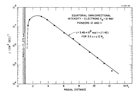
Fig. 5. An equatorial profile through the contours of Figure 4.
