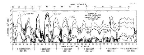
Fig. 7. Time dependences of the omnidirectional intensities of electrons in five different energy ranges during the Pioneer 10 outbound traversal of the outer magnetosphere on the dawn side of the planet.
