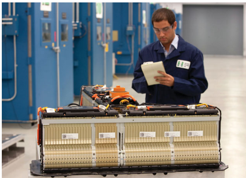
GM technician checks a lithium-ion battery pack for the Chevrolet Volt at GM's battery laboratory in Michigan.
