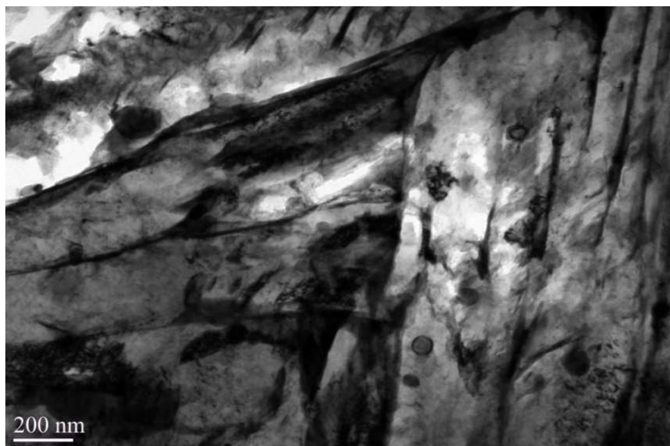
FIG 2: 200 kV TEM bright field image. Image shows precipitates within martensitic laths.
