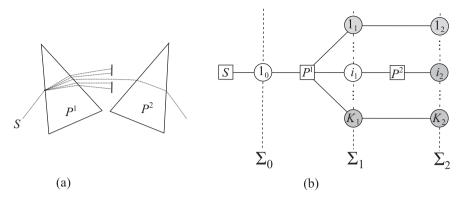
Figure 11.3. (a) Newtonian prism  $P^1$  splits an incoming beam of white light from source S (the Sun) into subbeams associated with primary colors. Prism  $P^2$  does not split any one of those subbeams further. (b) The QDN schematic of the same process.
