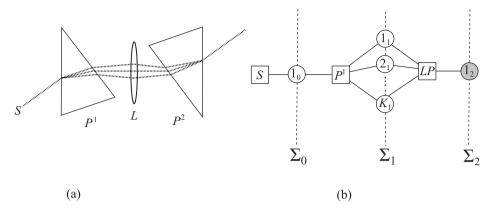
Figure 11.4. (a) Newton used lens L and prism  $P^2$  to recombine the spectrum from prism  $P^1$  back into a beam of white light. (b) In the QDN schematic of the same process, the lens and second prism constitute module LP.
